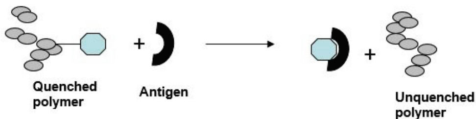
Figure 3. Removal of quencher by an antigen results in fluorescence
